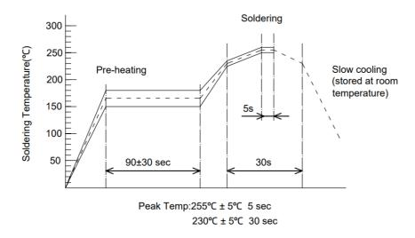
2. Recommended Soldering Parameters
